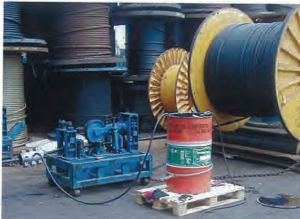
LubMasterGrease Application on Coiled Wire Ropes
