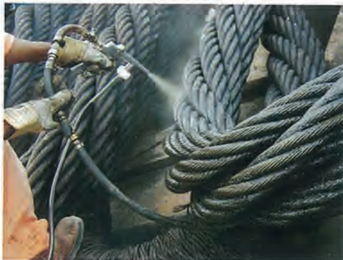
LubMaster WRD Cable Laid Application
